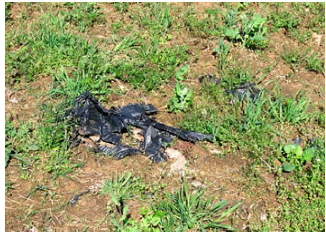
Photo 7. Pieces of pit liner lying in tilled area on the pad of 47-079-01200. Some pieces were firmly anchored in the ground, others were torn fragments lying loose on the surface. Photo taken 14 April 2011.
