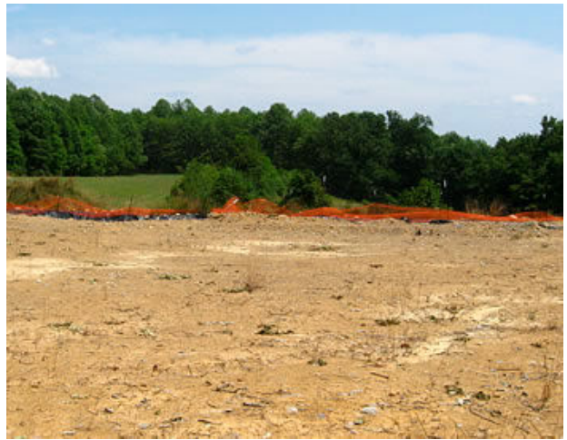
Photo 24. Pad bare of vegetation at 47-097-03716, plugged a year earlier. A soil sample collected at one of the lighter colored patches on the pad had chloride at 384 ppm. Photo taken on 1 July 2012.
