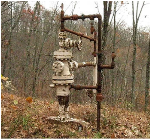
Photo 8. Wellhead 47-039-01168 showing leaking oily fluid below flange on casing head. Audible gas leak was heard here. Photo taken on 12 November 2012.
