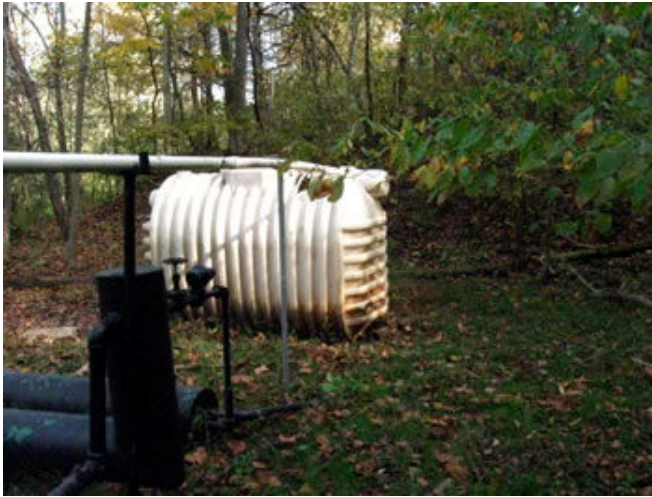
Photo 21. Condensate storage tank without secondary containment at 47-079-00615. This abandoned well lies just above South Poca River Road and is a short distance from the Pocatolico River. Photo taken on 12 October 2012.
