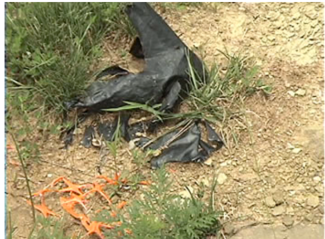
Photo 5. Large piece of exposed pit liner at 47-079-01314. Fragment of orange pit fencing is also visible. Photo from video shot on 7 June 2012.
