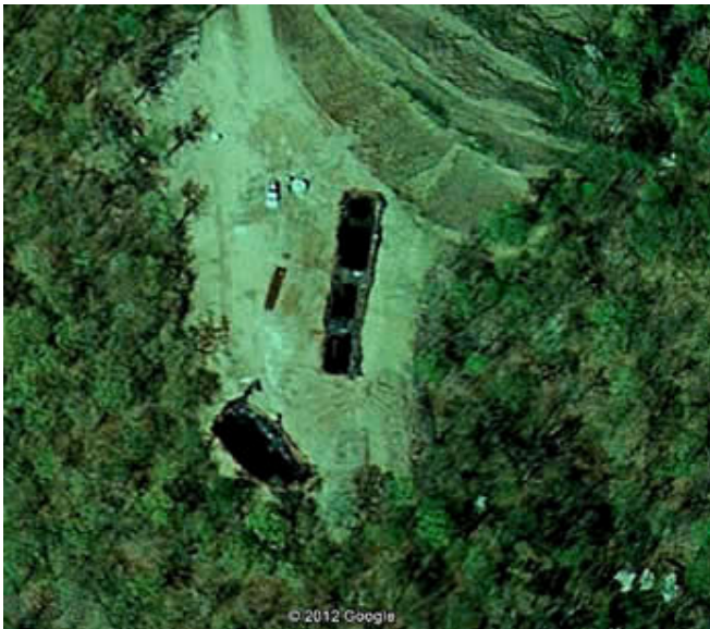
Photo 4. Satellite photo taken in 2005 of 47-079-01314. Line of exposed pit liner visible in 2012 is along western edge of large pit. Pieces of loose liner now lie on the surface near where the smaller pit is shown in the photo.
