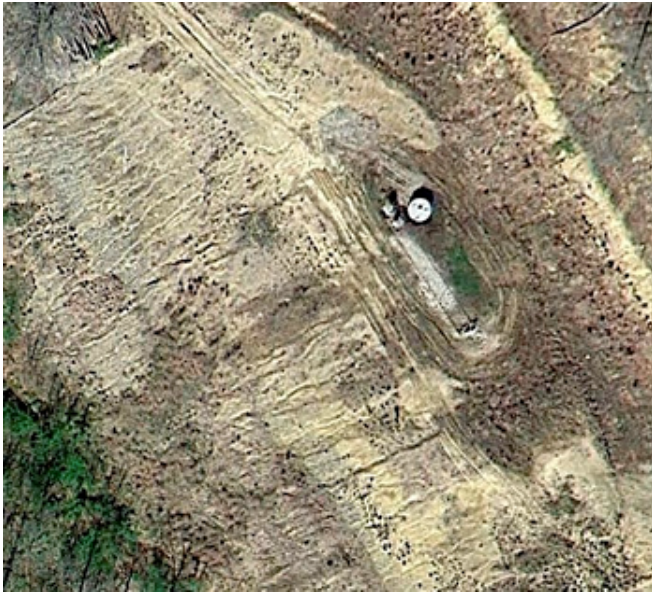
Photo 6. 26 March 2012 Google Earth image of 47-079-01324 in the Amherst Plymouth WMA. The large severely eroded fill slope takes up most of the left portion of the image. Google Earth imagery like this shows lack of secondary containment for tanks at wells in the WMA. Some sites like this have problems with slips and/or severe erosion.
