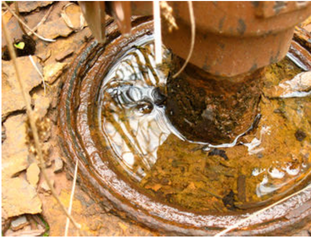
Photo 4. There are several small leaks on the heavily corroded casing head for 47-079-00748. Standing water was bubbling. Photo taken on 16 September 2013.
