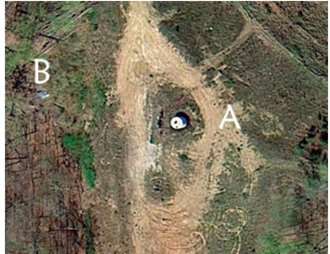
Photo 19. This is a 26 March 2012 Google Earth view of the pad for 47-079-01314 which shows vegetation coverage problems we found in 2012 and earlier visits. The letter A indicates the approximate location where samples showed high chloride in soil and surface water. The letter B shows the location of the blue portolet which has been pushed into the undergrowth away from the pad.
